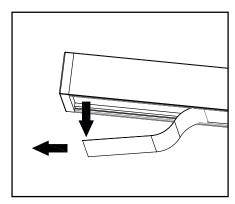
2. LGP (Light Guide Plate) removal. Utilizing the Extant Tool-Less Push & Eject System push on LGP approximately 4" from each end. You will notice the side closest to the led only moves a small distance. Continue pushing on the side opposite the LED until the LGP is released. You may have to push on the LGP several times to release it.
