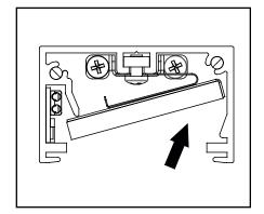
3. LGP installation. Insert LGP with the reflector side opposite the LED at approximately 45 degrees. Push LGP approximately 4" from each end to compress Tool-Less Push to Eject System and push towards LED. Push LGP several times up and towards the LED to ensure it is seated properly. Note: it helps to moisten fingertips slightly during this process.
