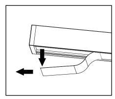
2. LGP (Light Guide Plate) removal. Utilizing the Extant Tool-Less Push & Eject System push on LGP approximately 4" from each end. You will notice the side closest to the led only moves a small distance. Continue pushing on the side opposite the LED until the LGP is released. You may have to push on the LGP several times to release it. Note: it helps to moisten fingertips slightly during this process.
