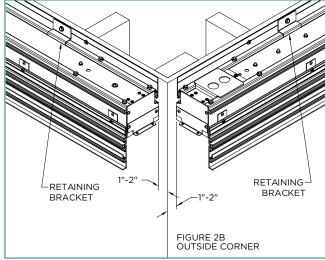
5. Use a framing square to measure from Fixture Extrusions to the intersection where they will meet (Figures 3A and 3B). Cut the Mitered Extrusions to these dimensions.
